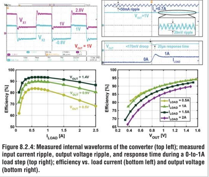
Figure 8.2.4: Measured internal waveforms of the converter (top left); measured input current ripple, output voltage ripple, and response time during a 0-to-1A load step (top right); efficiency vs. load current (bottom left) and output voltage (bottom right).
