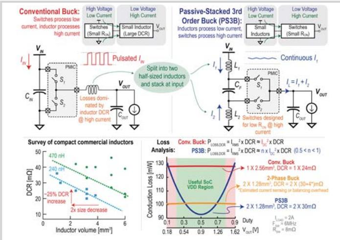
Figure 8.2.1: A conventional buck converter (top left) vs. the PS3B converter (top right) designed to operate small inductors, which have high DCR (bottom left), at the high-voltage low-current side of the converter to minimize conduction losses (bottom right).
