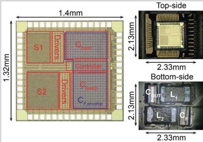
Figure 8.2.7: Micrograph of the fabricated stacked-passives 3<sup>rd</sup>-order buck converter (left); top side of the wirebonded prototype (top right); bottom side of the prototype (bottom right). The converter occupies 5mm<sup>2</sup> including the PMIC, passives, and the package area including the wirebonds and pads.
