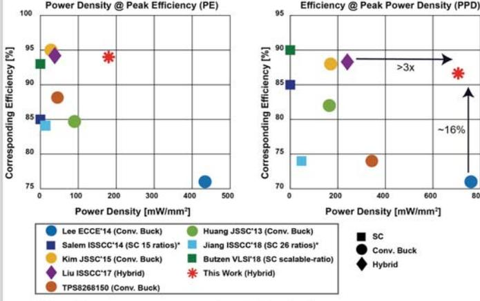
Figure 8.2.5: Measured efficiency and power density compared to prior-art converters that can efficiently regulate across SoC-compatible voltages and that report the total converter area (including the area of the passives and the interconnection between them).
