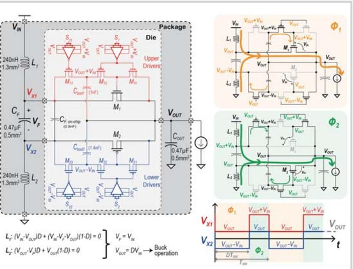
Figure 8.2.2: Schematic of the PS3B converter, along with associated timing diagrams.
