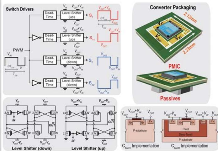
Figure 8.2.3: Generation of level-shifted signals from an input PWM signal (top left); level-shifter schematics (bottom left); 3D render of converter packaging (top right); bootstrap capacitor cross-section (bottom right).
