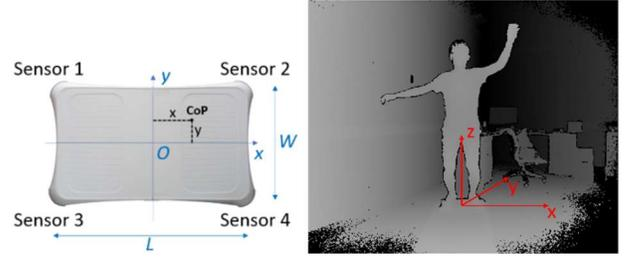
Fig. 3. Left: the WBB and its four pressure sensors. Right: the 3D coordinate system shown in the depth image.
