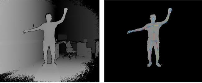
Fig. 2. Depth map captured by the depth camera of Kinect. Left: full depth map. Right: user depth map and the skeleton overlay.
