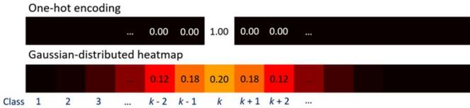
Fig. 6. One-hot encoding and Gaussian-distributed heatmap for the CoM ground-truth ( $k$  is the true class).
