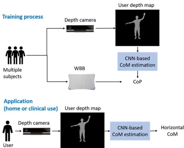
Fig. 1. The training and application process of the proposed CoM estimation framework.
