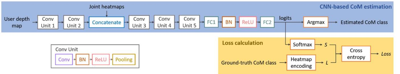
Fig. 5. The proposed network for CoM estimation.
