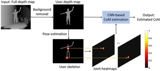
Fig. 4. The proposed CoM estimation Framework.
