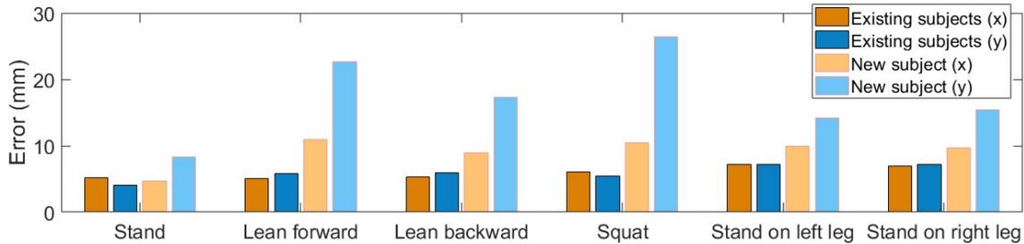
Fig. 7. The CoM estimation errors on different postures using our proposed approach.
