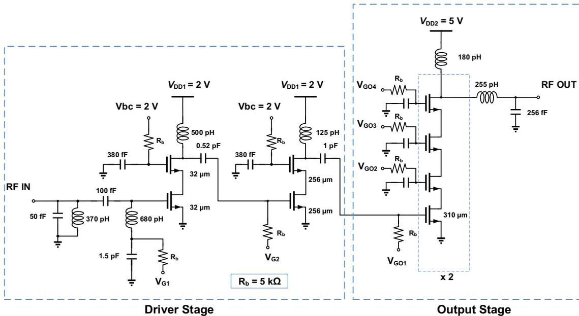
Fig. 2. The circuit schematic of the three stage multigate-cell stacked CMOS power amplifier.
