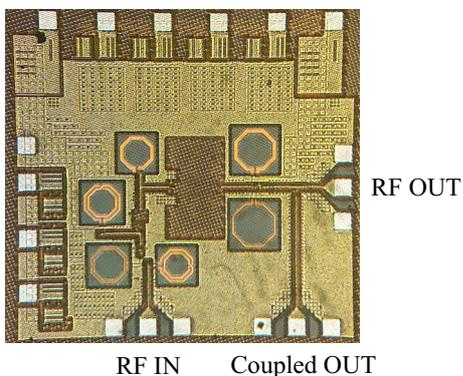
Fig. 3. Micrograph of the  $1 \times 1 \text{ mm}^2$ , three stage power amplifier chip.
