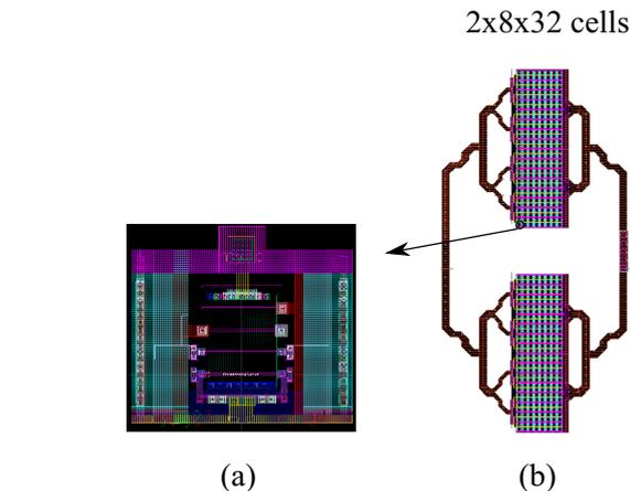
Fig. 1. (a) Layout of a single N-FET multigate-cell, (b) the final stage 2x256 cell device.
