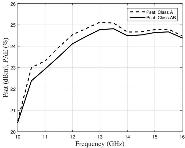
Fig. 6. Amplifier saturated output power  $P_{\text{sat}}$  vs. frequency for  $V_{G1} = 0.5$  V,  $V_{G2} = 0.3$  V, and final stage in class A ( $V_{GO2} = 0.45$  V) or Class AB ( $V_{GO2} = 0.3$  V.)
