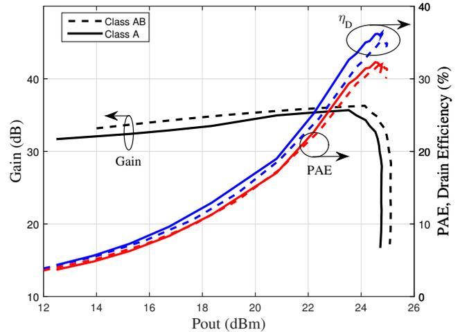
Fig. 5. Amplifier Gain, PAE and drain efficiency  $\eta_D$  vs. output power at 13.5 GHz for  $V_{G1} = 0.5$  V,  $V_{G2} = 0.3$  V, and final stage in class A ( $V_{GO2} = 0.45$  V) or Class AB ( $V_{GO2} = 0.3$  V.)
