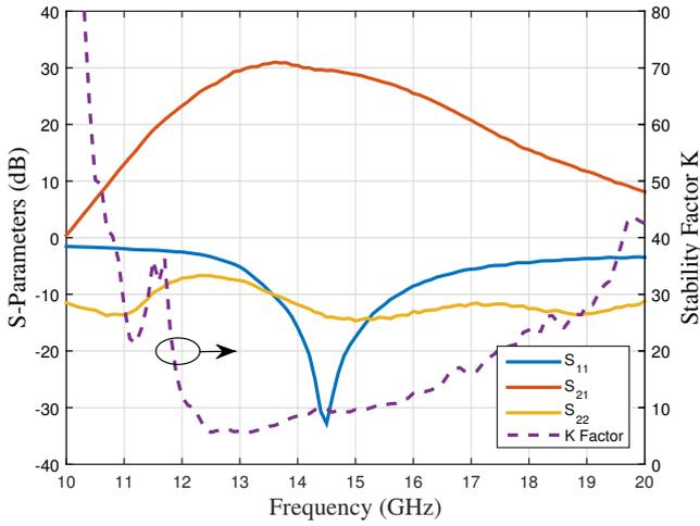
Fig. 4. Amplifier s-parameters for  $V_{G1} = 0.5$  V,  $V_{G2} = 0.3$  V, and  $V_{GO2} = 0.45$  V.
