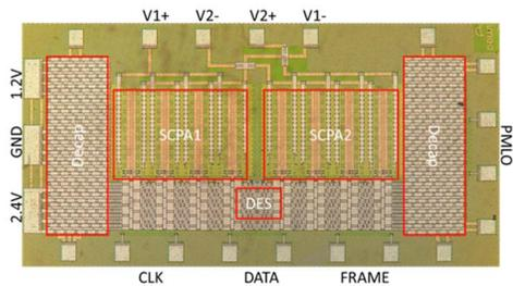
Fig.6. Chip Micrograph (1.8mm x 0.9mm)
