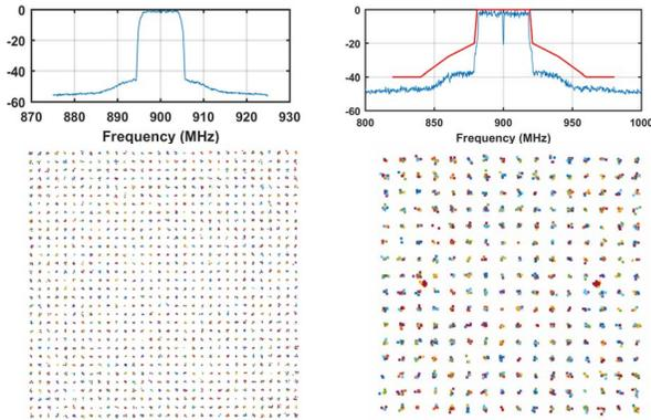
Fig.10. Left: Measured spectrum and constellation of 9 MHz 1024-QAM OFDM modulation. Right: Measured spectrum and constellation of 40 MHz 256-QAM 802.11ac modulation.
